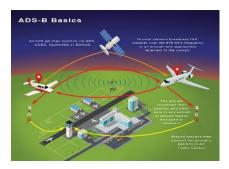
Without describing every detail ADS-b OUT sends a signal from the aircraft which is received by a ground-based station and is relayed to ATC. This information includes the airplane N, altitude and vertical speed. The ground station then transmits the ADS-b IN signal in response. ADS-b IN is the complementary function in
