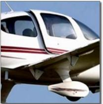
While the opening of the door is startling when it happens, you should not let it worry you. The picture above shows the maximum amount the door will open in flight. Wind pressure will hold it in this position.
