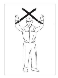
Once you stop you should shut down the engine. At some airports the marshaller may then place chocks on some of the wheels. Make sure you are providing a safe environment for them to do this. When I stop my engine, I will remove the key and hold it up so the marshaller may see it as a confirmation that I have made the propeller area safe.
